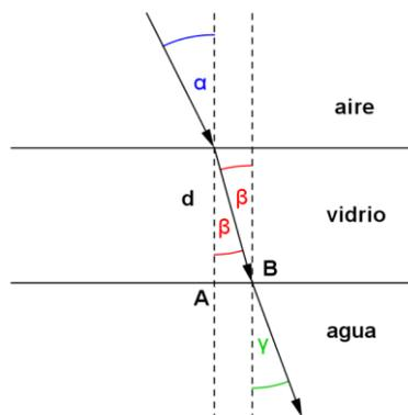
b)  $\text{tg } \beta = \frac{AB}{d}$   $AB = d \cdot \text{tg } \beta = 30 \cdot \text{tg } 18,21^\circ = AB = 9,87 \text{ mm}$
