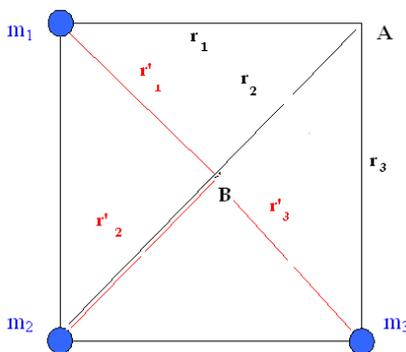
$$V_A = -G \frac{m_1}{r_1} - G \frac{m_2}{r_2} - G \frac{m_3}{r_3} = -Gm \left( \frac{1}{r_1} + \frac{1}{r_2} + \frac{1}{r_3} \right)$$
